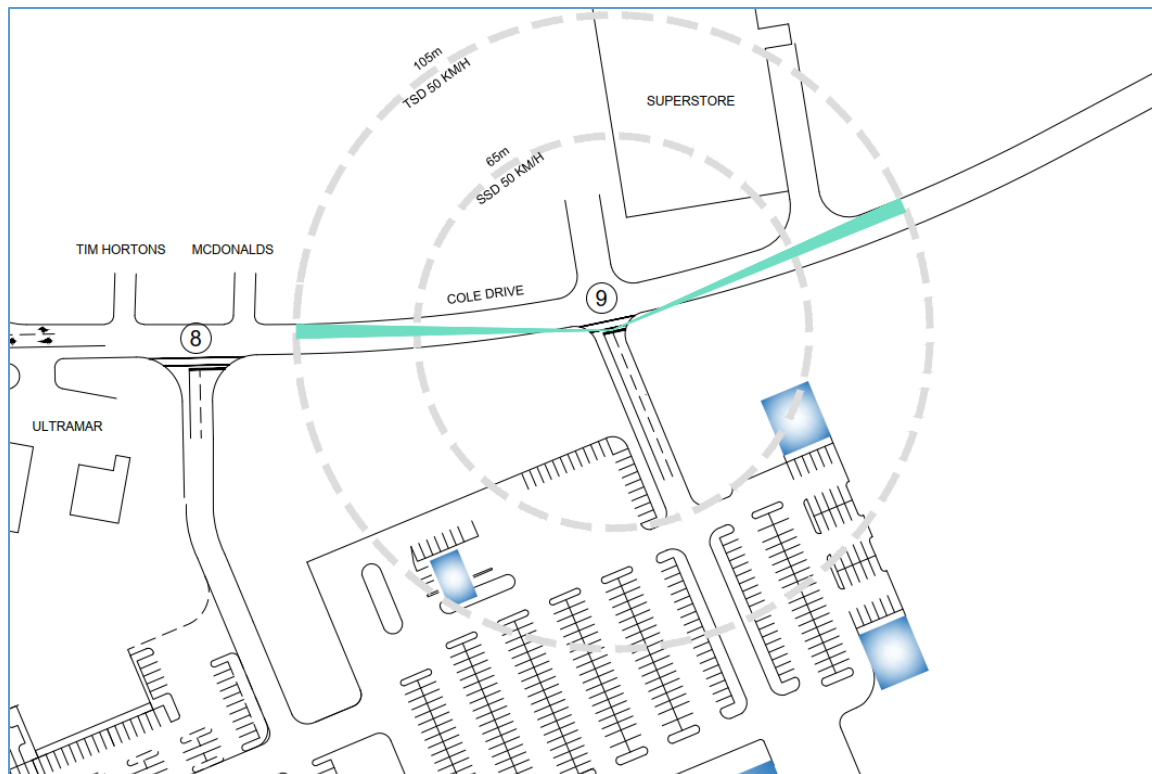
Figure 12 - Sight Distance for Driveway #9
