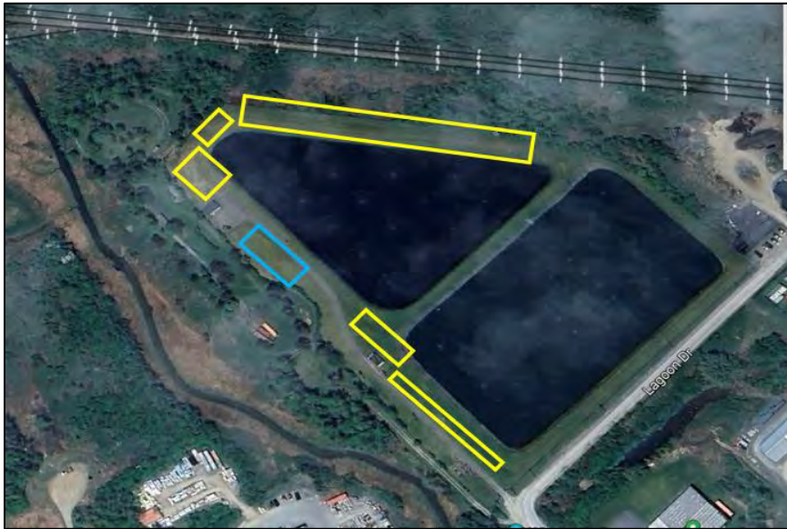
Figure 6.6: Ortho - 3 Lagoon Drive - Ballasted PV array area (yellow), anchored PV array (blue) (GoogleEarth, 2024)
