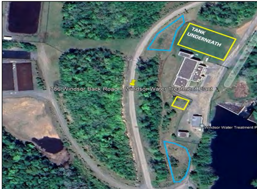
Figure 7.7: Ortho – 786 Windsor Back Road - Ballasted PV array area (yellow), anchored PV array (blue) (GoogleEarth, 2024)
