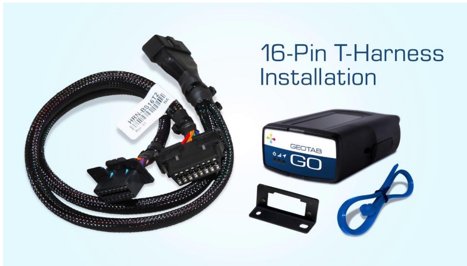
Figure 1: OBD-II device (right) and harness (left) used in the Taking the Wheel study.
