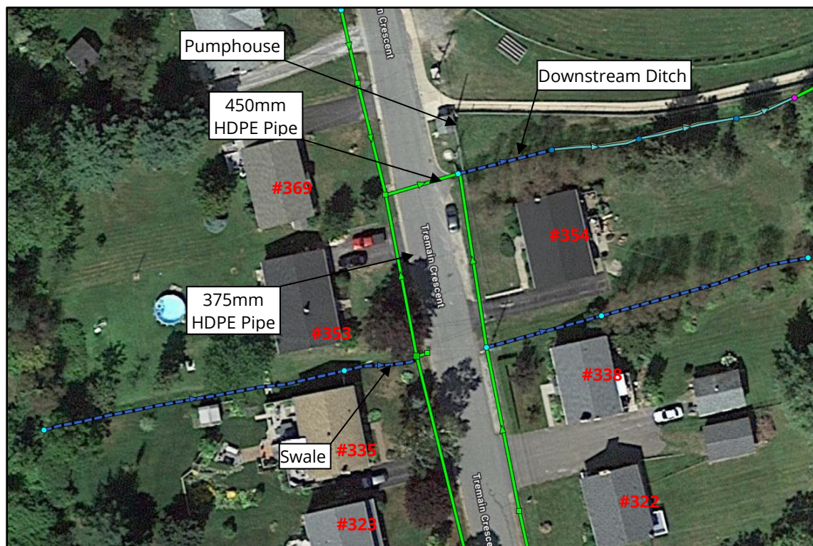
Figure 1: Tremain Crescent – Storm Sewer Infrastructure near Civic #335
