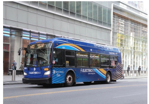
Figure ES-2: 35ft Urban Transit Battery-Electric Bus
