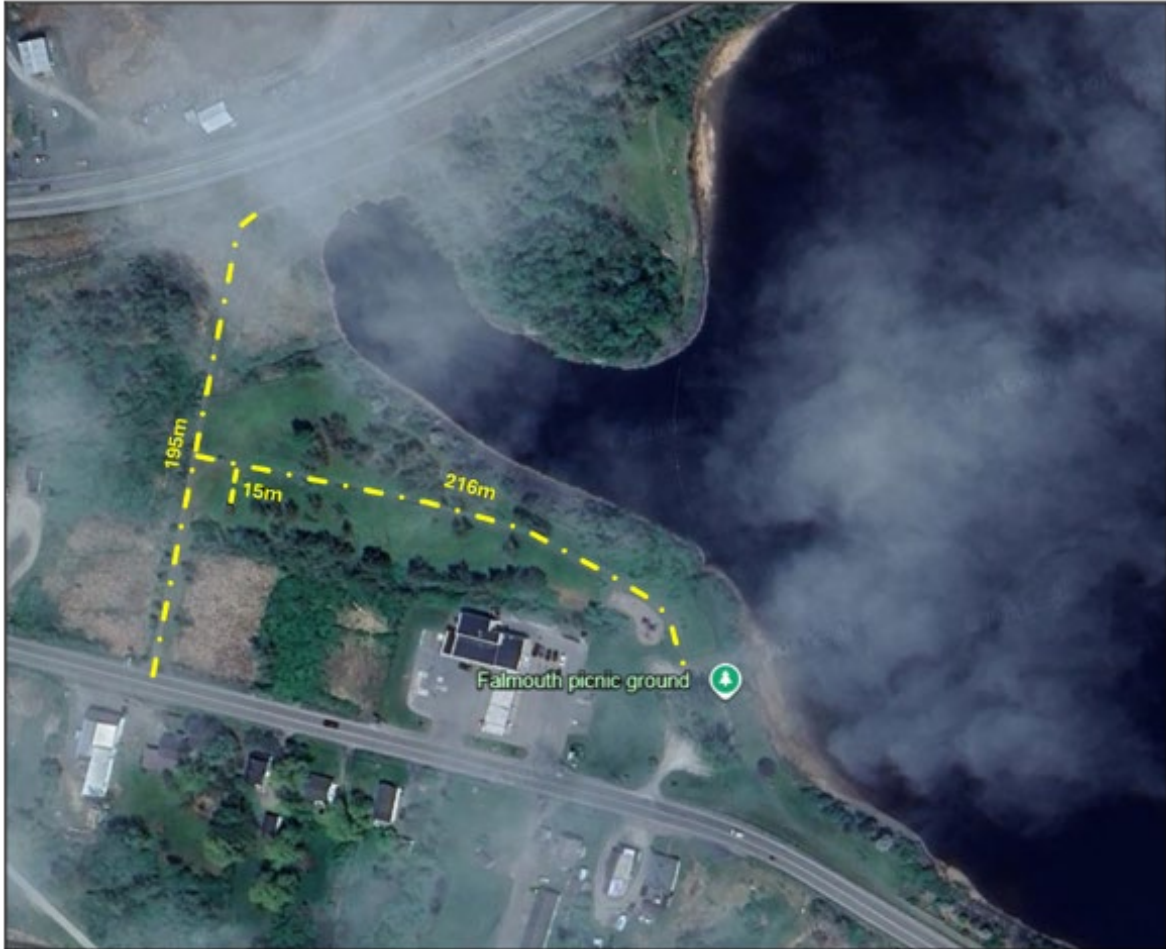
Figure 1. Replacement Sections Along Falmouth Causeway Trail
