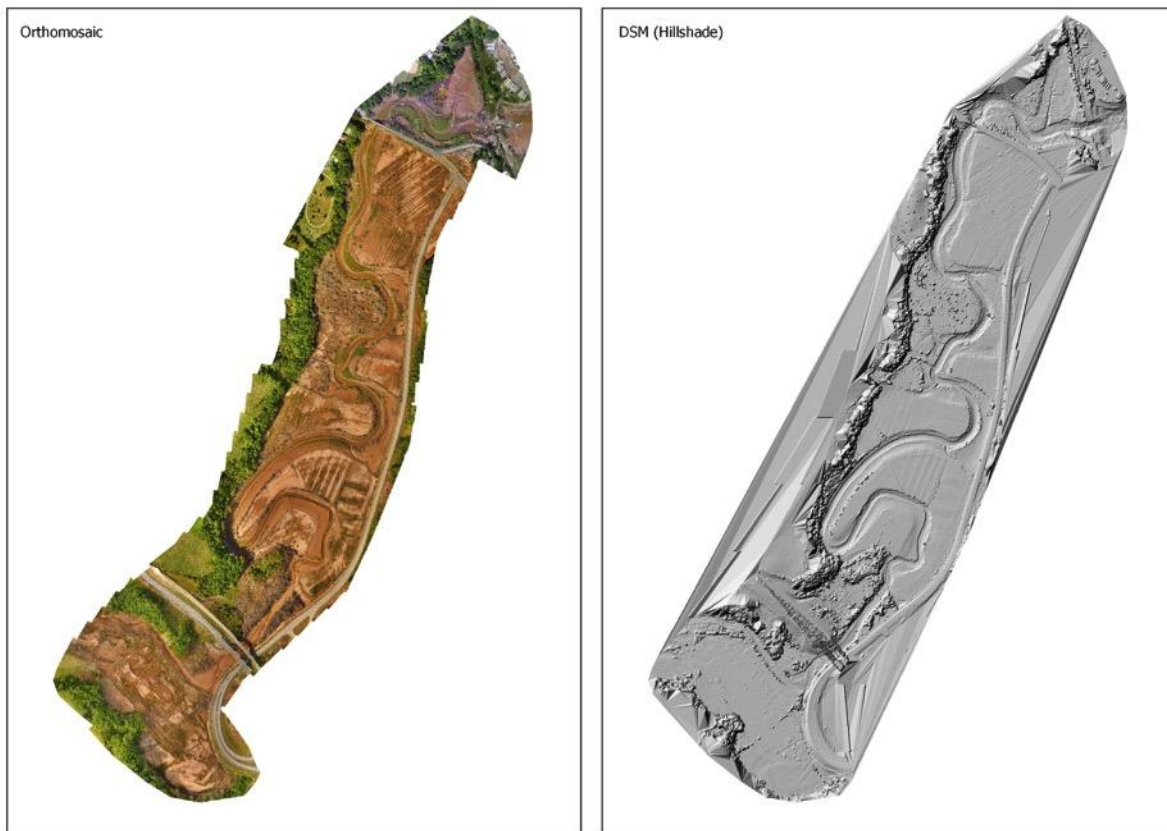
Figure 6 Orthomosaic and DSM derived from the georeferenced low-altitude aerial photography.
