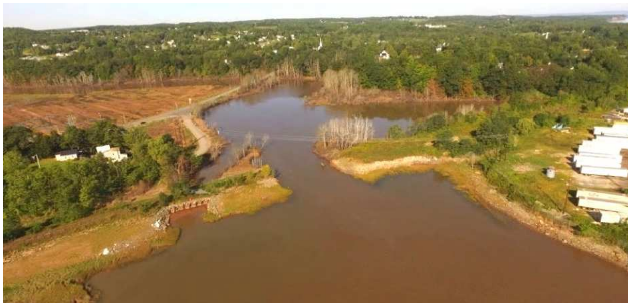
Figure 4: Aerial photograph of mouth of the Halfway River and breach site. Photograph was taken at high (neap) tide on September 5, 2018. The secondary, overflow, aboiteau is to the left of the main opening. Drone imagery by CBWES 2020.
