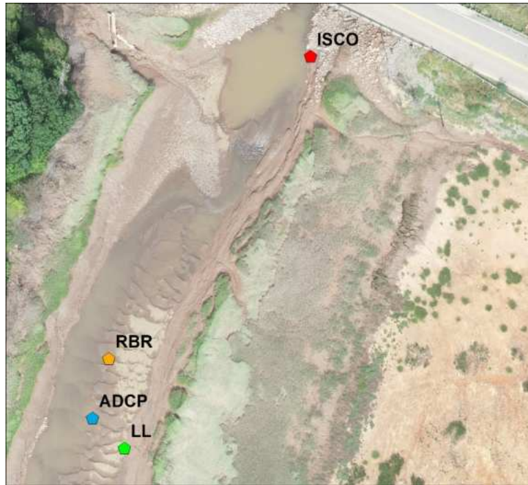
Figure 24: Aerial view of location of instruments deployed to measure SSC, velocity, water levels, turbidity and salinity, during July 2019 deployment. Similar sampling locations were used in 2020.
