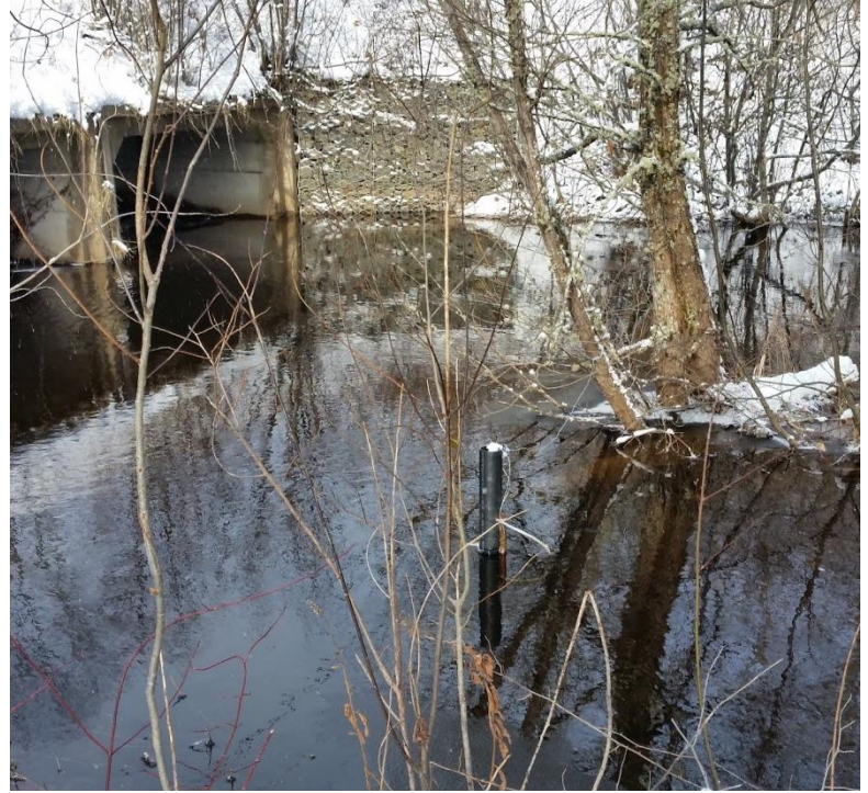
Figure 3-3: Water Level Logger 2 (LL2) installation
