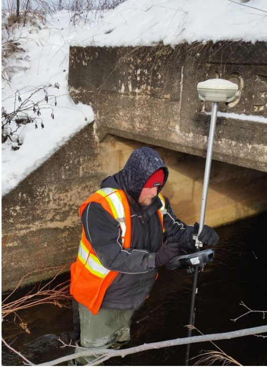
Figure 3-2: Surveying the water level logger
